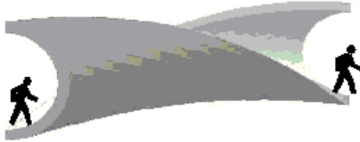
Swept C-shaped cross section with a longitudinal twist of 180° also offers a level walking surface.
